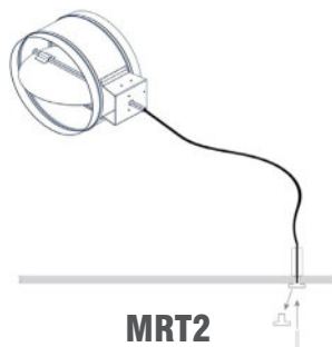
Manually operated damper, cable through drywall with termination fixture
