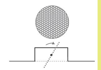
**IMPORTANT**: the perforated damper also acts as an air equalizer. Therefore if there is an angle in the duct entering the plenum, please make sure that the flat part of the damper is always facing the angle of the duct when possible. This will help ensure optimal air equalizing.
