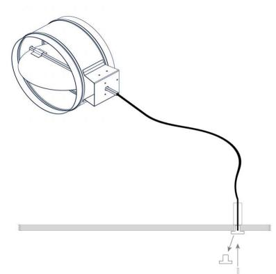
5. Support cables as required at all changes in direction and at 3 foot intervals. Use retaining clips furnished. NO DRAPING – cables should be taut or nearly so. 4" minimum turn radius. Clips should be installed with a loose fit to allow cable rotation. The longer the cable and the larger the damper – the more attention should be paid to cable support.
