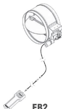
Battery operated electro-balance damper with remote control, cable through drywall with termination fixture
