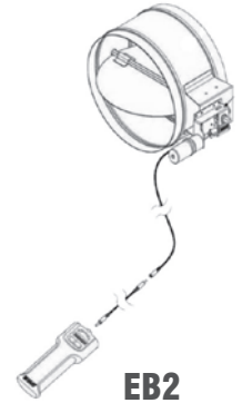
EB2 Battery operated electro-balance damper with remote control, cable through drywall with termination fixture
